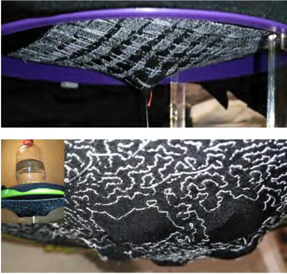
**Figure 7: Results showing qualitative response of embroidered samples. Top: Target example with EB approach shows graded stiffness toward center of target. Bottom: Waterbottle cushion shows how stiffening contours and redistributes pressure under load.**
