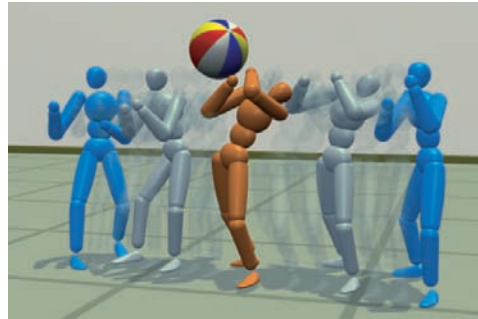
Figure 1: An example anticipation pose. The blue poses represent motion capture frames, grey poses represent interpolation frames, and the orange pose represents the character’s pose at impact.
