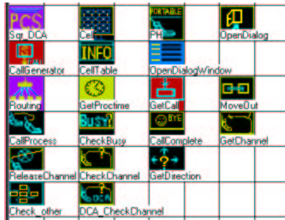
Figure 6: Extending the model . The top row of the figure contains an icon for the square network using the dynamic channel allocation scheme ( Sqr_DCA ). The icon DCA_CheckChannel , shown in the bottom row, is a method derived from Check_Channel ; DCA_CheckChannel extends the functionality of Check_Channel .
