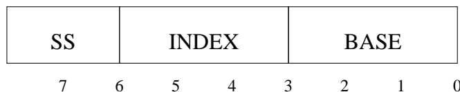
Figure 6: SIB byte . The SIB byte consists of a 2 bit scale field, a 3 bit index field, and 3 bit base field. It specifies the based indexed and scaled indexed forms of 32-bit addressing.
