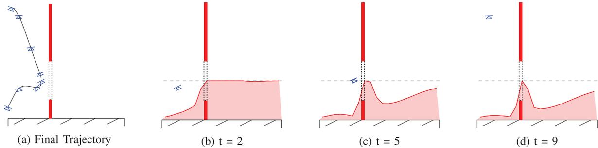
Fig. 5. A **closed window**. Red rectangles are opaque obstacles, while the dashed box is a transparent obstacle. (a) Our C-OPT Path (b)-(d) the evolution of the uncertainty (the filled region) over time. Dashed line shows the initial region uncertainty.
