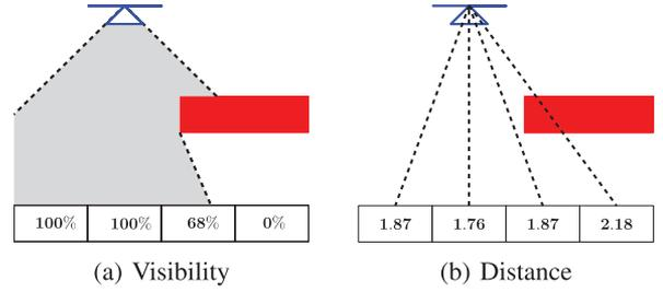
Fig. 1. **Modeling the viewing uncertainty of a region.** The robot accounts for (a), the visibility, by calculating what percentage of the region is within its field of view (the gray shaded region) and not obstructed by obstacles (the red rectangle). The robot also accounts for (b), the distance from the center of the region to the robot.
