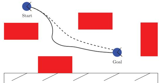
Fig. 6. **Point-To-Point Optimization**. The dashed line shows the collision-free trajectory, while the solid line shows our C-OPT trajectory. The red rectangles are the obstacles (desks in the lab). Planning with our approach provides good views of the entire target wall.
