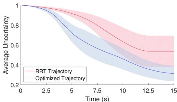
Fig. 8. **Optimized path quality comparison.** The red line shows the average region uncertainty over the collision-free planning path. The blue shows the results using C-OPT. Shaded regions denote the respective 95% confidence intervals. The C-OPT trajectory enables the robot to see much more of the lab’s wall, resulting in significantly less uncertainty.
