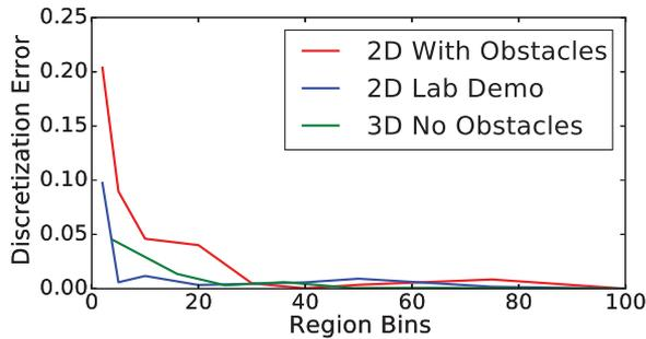
Fig. 10. **Coverage quality for various discretizations.** The lines show the effect of increasing the region discretization on the average uncertainty of the optimized trajectory. The region uncertainty for each discretization is compared to the uncertainty obtained planning a path where the region is discretized into 200 bins. As  $k$  increases, the coverage quality of the path converges.
