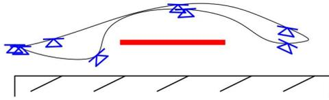
Fig. 9. **Planning with spatially varying uncertainty.** A localization beacon is placed at the starting position on the left. Positional sensing quality decays the further the robot is from the beacon. The robot plans a path that stays further from the obstacle when it is less certain about its position.
