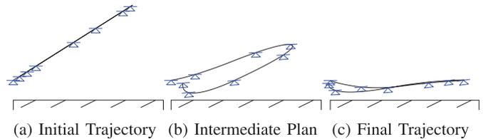
Fig. 2. **Evolution of initial trajectory over iLQG iterations.** Each iteration reduces the overall cost function (Eq. (4)) and improves the planned path.
