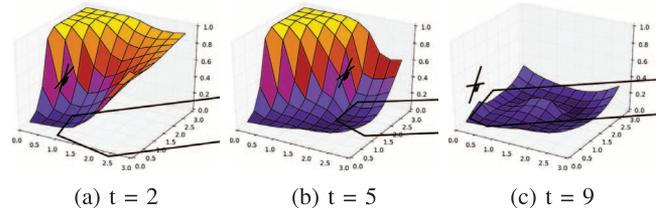
Fig. 3. **3D coverage planning with acceleration controls.** Region uncertainty is shown at time  $t = 2, 5$ , and  $9$  seconds. The black quadrilateral represents the area the robot can see from its current state. The planned path successfully observes the entire region.
