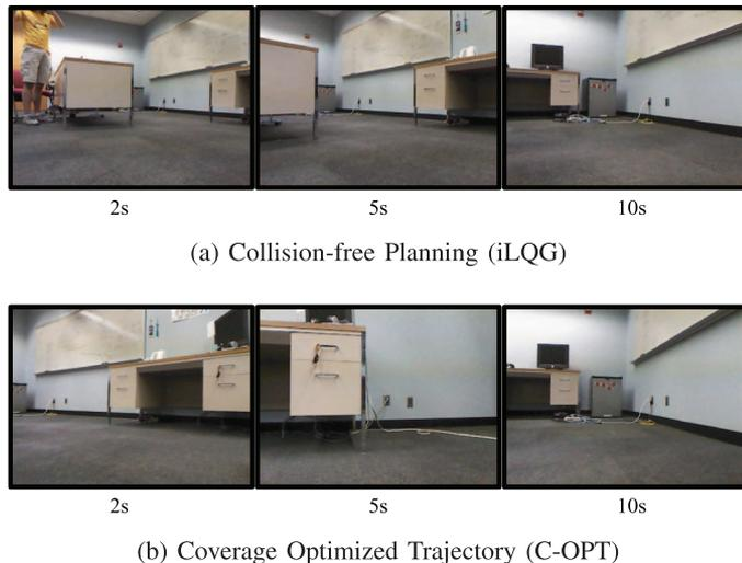
Fig. 7. **Implementation on a robot.** First-person view from the onboard camera of the robot as it executed both the collision-free plan and the C-OPT trajectories. In the 5s image, the coverage-optimized trajectory is able to see the wall on the right side of the desk.
