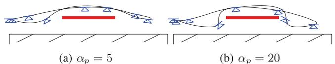
Fig. 4. **Effect of uncertainty cost parameter.** An omni-directional, acceleration controlled robot attempting to sense the floor. The rectangle is an opaque obstacle. We show the optimized path for two different weights of the uncertainty cost ( $\alpha_p$ ). As the uncertainty weight increases, the path becomes much more aggressive in getting to optimal views.
