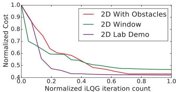
Fig. 11. **Cost over iLQG iterations.** The cost over iterations for each of the scenarios is shown. Costs quickly decrease at first, and then converge to a locally optimal value. The costs for each scenario are normalized based on the cost of the initial trajectory. The iLQG iterations for each scenario are normalized based on the total number of iterations it took to run each scenario.
